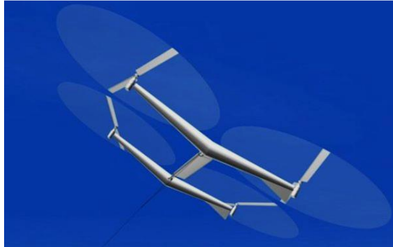
Figure 6 Rotorcraft airborne wind turbine concept. Adapted from [11]
