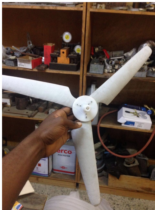
Figure 19 Picture of blade support with the rotors mounted on it
